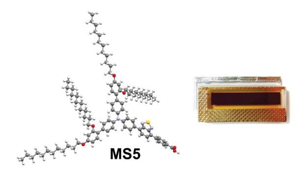
3D structural representation of MS5 and photograph of 3.8 cm2-size dye sensitized solar cells. Credit: Marko Stojanovic and Dan Zhang
