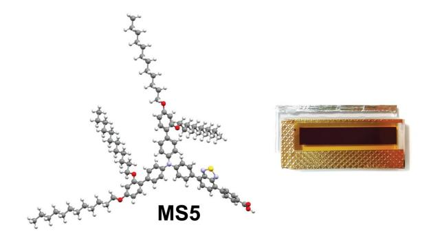
3D structural representation of MS5 and photograph of 3.8 cm2-size dye sensitized solar cells. Credit: Marko Stojanovic and Dan Zhang
