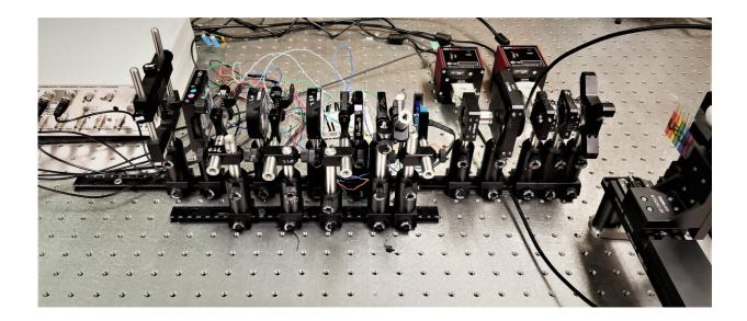
Inspired by the eyes of mantis shrimp, researchers developed an optical sensor that is small enough to fit on a smartphone but is capable of hyperspectral and polarimetric imaging. This photo shows an experimental prototype of the sensor. The tandem structure consists of 6 polarization-sensitive organic photovoltaics and 4 polymer retarder films cascaded in series along the same optical axis. Credit: Ali Altaqui
