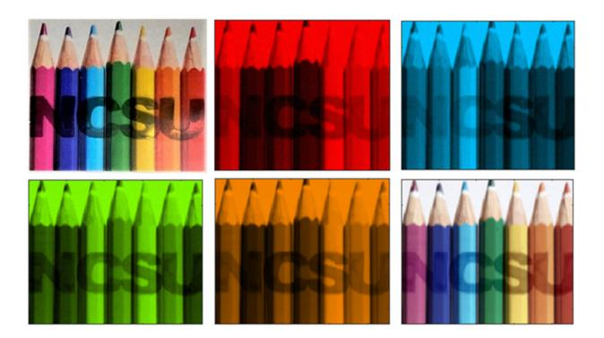
Inspired by the eyes of mantis shrimp, researchers have developed an optical sensor that is small enough to fit on a smartphone but capable of hyperspectral and polarimetric imaging. This image shows spectral imaging of a scene containing objects with different colors, as well as the letters NCSU, which contain different polarization states. Credit: Ali Altaqui
