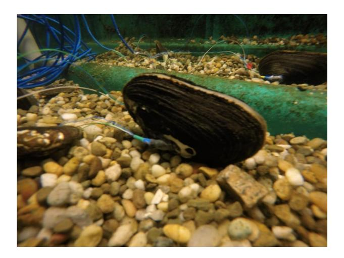
Researchers at North Carolina State University have designed and demonstrated a new system that allows them to remotely monitor the behavior of freshwater mussels. A prototype of the system is shown here. The system could be used to alert researchers to the presence of toxic substances in aquatic ecosystems. Credit: James Reynolds, NC State University
