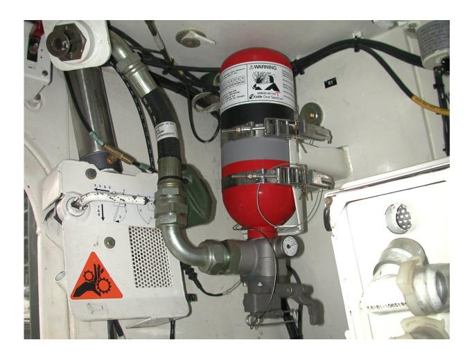
The U.S. Army uses NIST's PROFISSY computer program to help understand the performance and calculate the maximum charging pressure for this automatic fire extinguishing system, which protects the crew in an armored ground vehicle from explosive fires. Credit: U.S. Army
