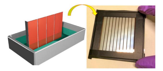
A new dipping process using a sulfolane additive creates high-performing perovskite solar cells. The method is inexpensive and well-suited for scaling up to commercial production. Credit: Los Alamos National Laboratory
