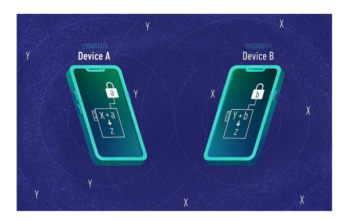
NIST researchers developed a cryptographic system using encounter metrics. Encounter ID is a way of labeling an encounter between two people through a random number not linked to the device each person carries. To generate the randomized number Z, each device calculates using their private info (a and b) and what the other device is broadcasting (X and Y). Cryptography ensures that device A's Z is the same as Device B's Z. Credit: B. Hayes/NIST
