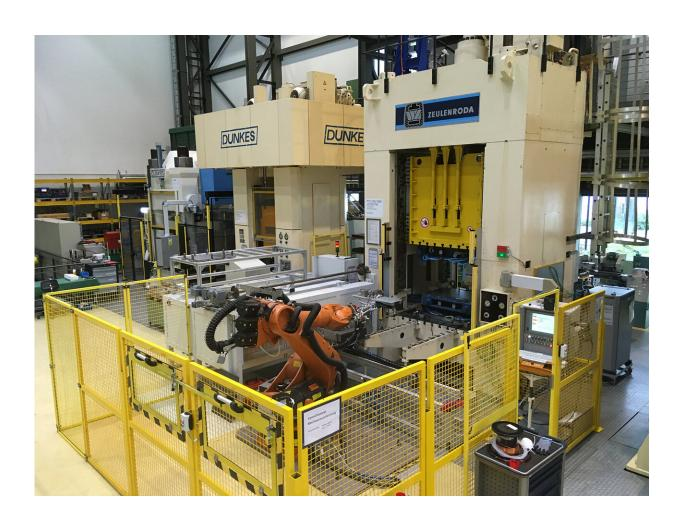
Test rig for hot sheet metal forming at Fraunhofer IWU, including oven, press, and robot. Credit: Fraunhofer-Gesellschaft
