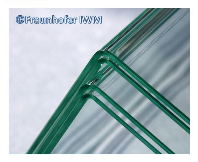
The results of the glass-bending process: glass panes bent at a 90° degree angle. Credit: Fraunhofer-Gesellschaft
