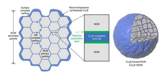
Schematic coating-plus-infusion microstructure in which CoxB uniformly coats the surface of NCM secondary particle and infuses into GBs between the NCM primary particles. Credit: Ulsan National Institute of Science and Technology
