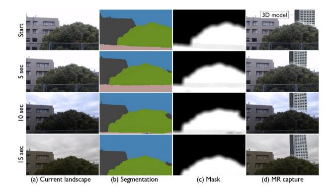
Fig. 2 MR-based landscape visualization with dynamic occlusion handling in field validation. Credit: Osaka University
