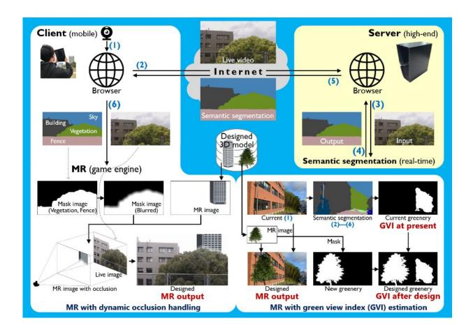
Fig. 1 Proposed MR system: Integration of semantic segmentation into MR. Credit: Osaka University
