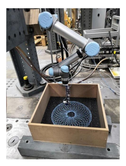
The robotic arm lays out the "knitting pattern." Empa researchers are investigating different patterns in a number of test series. Credit: Empa
