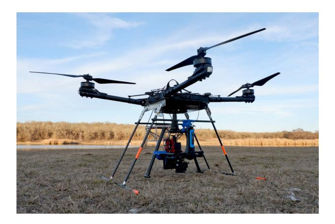
Aerial robots developed by UT Dallas researchers can carry several cameras, an array of onboard sensors and a downwelling irradiance spectrometer — all used to gather data for mapping and to learn the characteristics of environments. Credit: Lakitha Wijeratne/UT Dallas physics doctoral student
