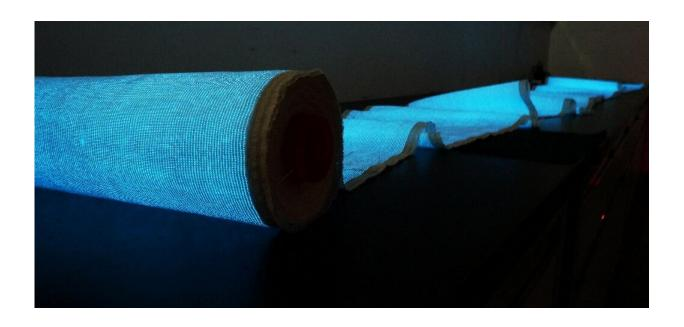
The wearable, foldable and washable fabric is capable of flashing messages or images
