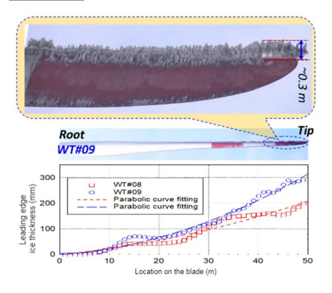
How ice builds up on the tips of turbine blades. Credit: <u>Gao, Liu and Hu, 2021</u>, <u>CC BY-ND</u>
