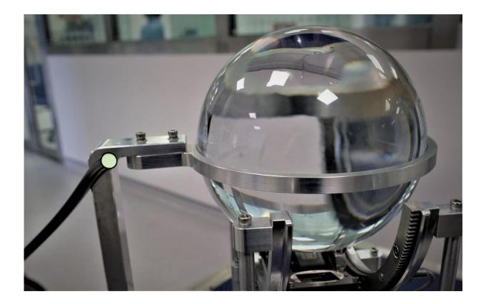
The acrylic ball (right) of the device acts as the solar concentrator, enabling sunlight to form a sharp focus. The focused sunlight is then collected into one end of a fibre cable (left) and emitted via another end directly. Credit: NTU Singapore
