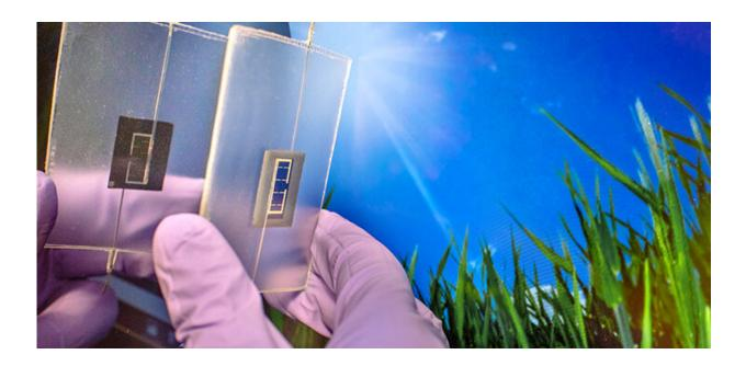
The efficiency of solar cells can be increased by combining two light-absorbing materials. Such tandem devices derive energy from both direct sunlight and light reflected from other surfaces. Credit: KAUST; Anastasia Serin
