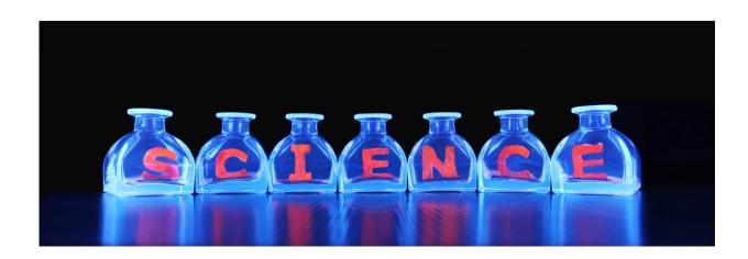
Demonstration of an 'impossible bottle' construction. Drawing on thin and flexible film enables on site reconfiguration of a 3D architecture inside a narrow space that would be inaccessible to conventional 3D pr inters. Credit: Song et al., Sci. Adv. 2021; 7: eabf3804
