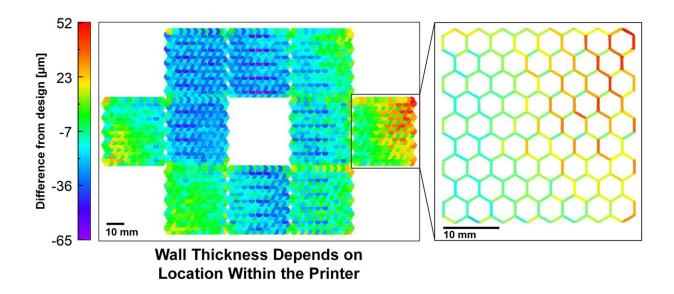
The software can detect defects in the printed parts and determine where in the printer the defects occur. Credit: University of Illinois Urbana-Champaign
