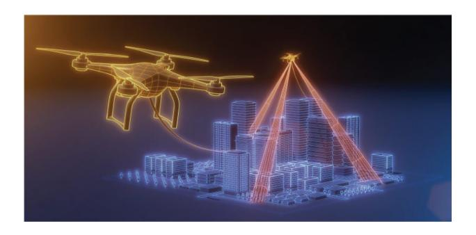
Wireless connectivity in temporary high-usage hotspots, such as where large crowds gather, could be enhanced using tethered drones connected to a ground station. Credit: KAUST; Xavier Pita
