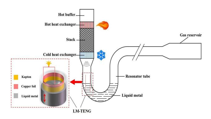
Schematic of a thermoacoustically driven liquid-metal-based triboelectric nanogenerator. Credit: Shunmin Zhu, Guoyao Yu, Wei Tang, Jianying Hu, and Ercang Luo
