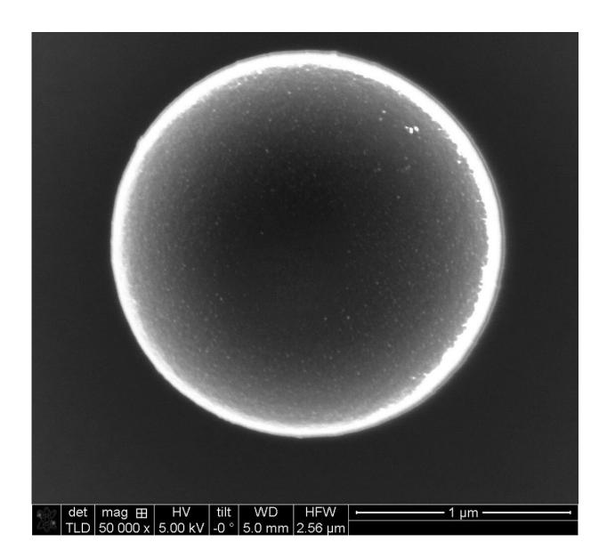
Electron microscope image of a microswimmer. The particle is 2.18 micrometres in diameter. The small, brighter dots on the particle are gold
