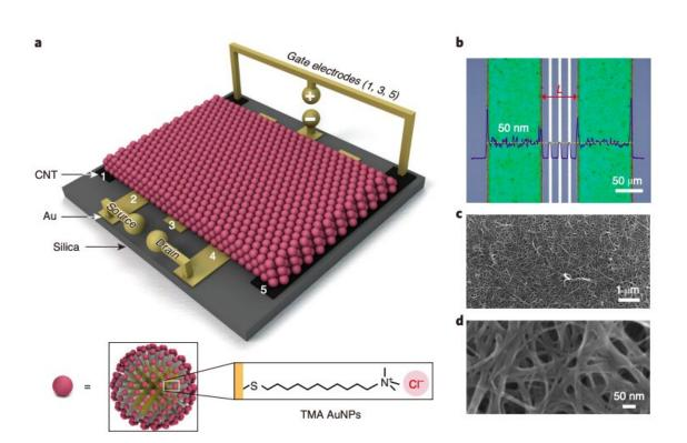
Schematic and experimental images outlining the design of the metal nanoparticle film-based transistor created by the researchers. Credit: Zhao et al.
