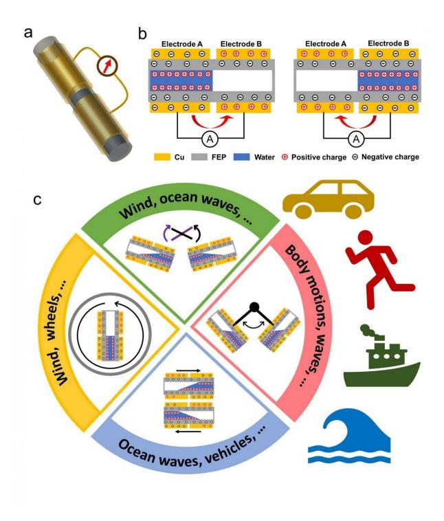
The team encapsulates water in a finger-sized tube. When water moves in the tube between regions of the two electrodes, triboelectrification happens and electric currents can be generated. Taking advantage of the flexibility of water, the WT-TENG can be operated in various modes, including rotation, swing,
