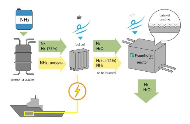
Ammonia is split into nitrogen and hydrogen in the ammonia cracker. The latter is then burned in the fuel cell to generate electric-ity. The catalytic converter ensures that no harmful nitrogen oxides are produced. The only end products are water and nitrogen. Credit: Fraunhofer
