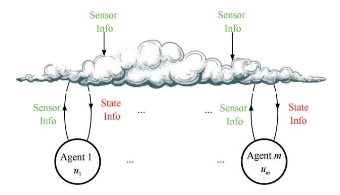
Conceptual struture of a multiagent system. Each agent is supplied a "state info" from the "cloud" at each stage of decision making, which then performs local computations based on this state information to apply their controls. Credit: IEEE/CAA Journal of Automatica Sinica, Image courtesy: Dimitri Bertsekas
