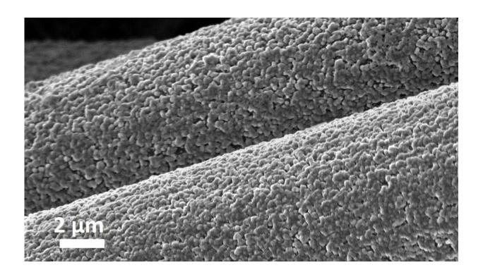
This magnified image shows aluminum deposited on carbon fibers in a battery electrode. The chemical bond makes the electrode thicker and its kinetics faster, resulting in a rechargeable battery that is safer, less expensive and more sustainable than lithium-ion batteries. Credit: Cornell University
