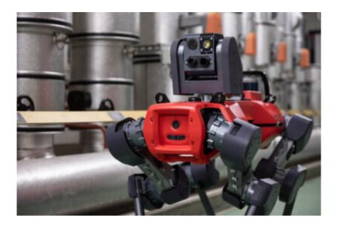
The pan-tilt inspection unit features high-end sensors for accurate and reliable visual, thermal, and acoustic measurements. Credit: ANYbotics
