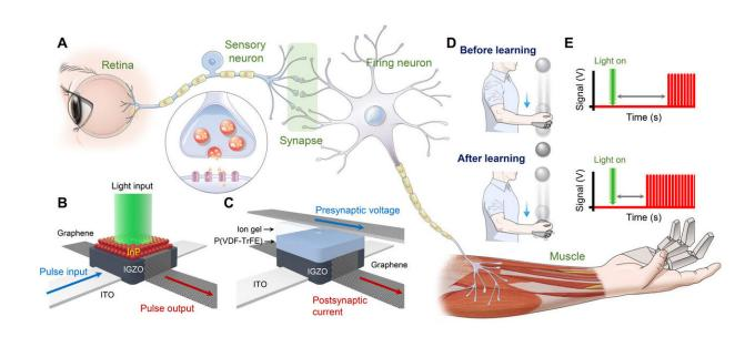
Artificial stimulus-response system. (A) Schematic illustration of biological stimulus-response system composed of retina, neurons, synapse, and muscle. (B and C) Schematic device structure of (B) AVR with InP QD layer and (C) AS with retentive EDL. (D) Schematic illustration of a human individual catching a ball successfully through learning. (E) Neural signals before and after learning process. Credit: *Science Advances* (2021). DOI: 10.1126/sciadv.abe3996
