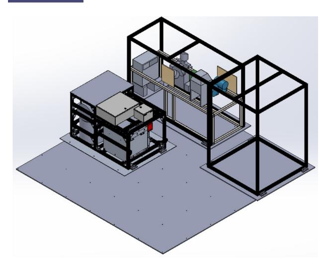
A team of engineers has built three experiments to test the effects of microgravity on a new oil-free fridge design: a prototype for potential future use on the International Space Station (left), a setup for testing the prototype's vulnerability to liquid flooding (center), and a larger version of the prototype with sensors and instruments to capture how gravity affects the vapor compression cycles (right). Credit: Air Squared, Inc.
