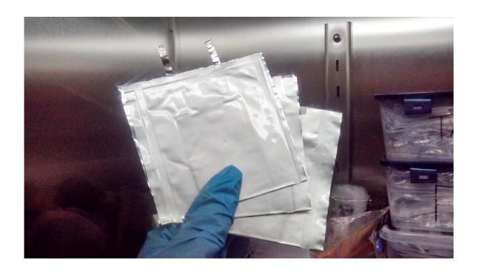
Electrodes removed from the batteries. Electrodes consist of a film made from aluminum or copper, for example, which is covered with a thin layer of active material. Photo: Aalto University Credit: Aalto University
