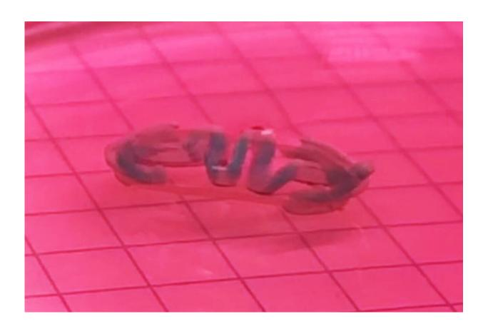
Side view of a swimming biobot developed at IBEC, consisting of a muscle cell-laden hydrogel and a spring-like skeleton. These biobots can self-train, showing surprising speed and strength. Credit: IBEC
