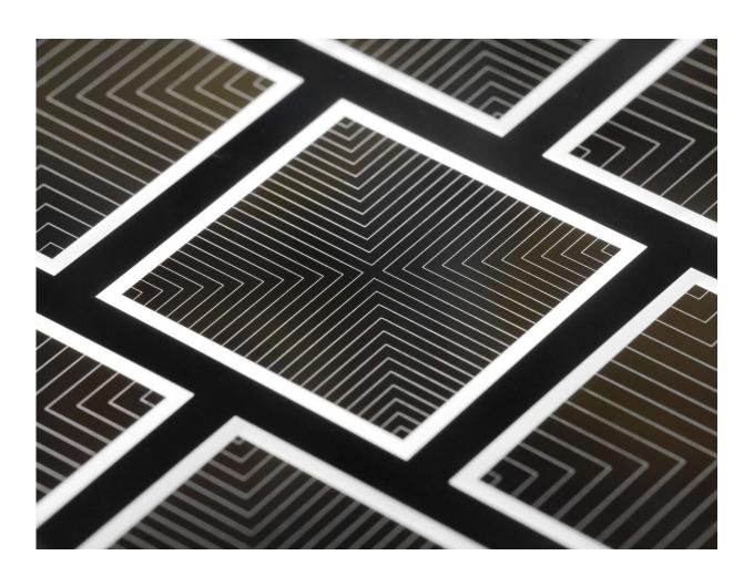
The TOPCoRE solar cell achieved 26 percent efficiency, a new world record for both-sides-contacted solar cells. Credit: Fraunhofer-Gesellschaft
