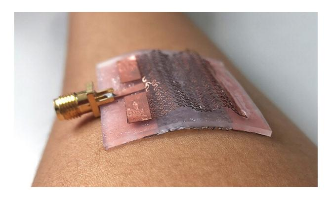
The wearable transmitter is designed to compress its top layer in a double arch pattern, shown here, to respond to movement without compromising signal transmission. Credit: Huanyu Cheng, Penn State
