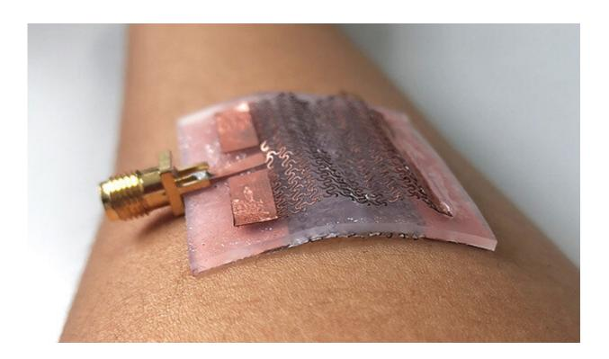
The wearable transmitter is designed to compress its top layer in a double arch pattern, shown here, to respond to movement without compromising signal transmission. Credit: Huanyu Cheng, Penn State
