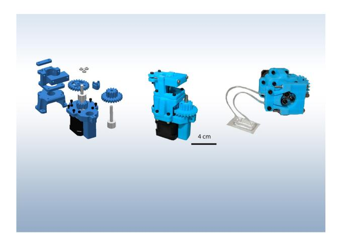
The pump is assembled with a combination of 3D-printed parts and commonly available hardware, and is programmable via an Arduino microcontroller. Credit: *Scientific Reports* DOI: 10.1038/s41598-020-58246-6.
