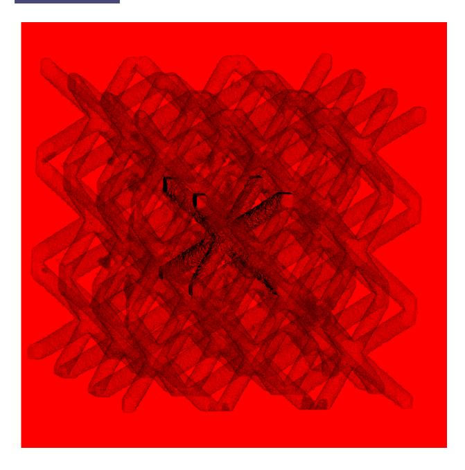
Following the example of avian bones, intricate lattice structures inside of hollow turbine buckets provide the necessary stability. 3D-image of the lattice structure reconstructed from x-ray tomography data. Credit: Dr. Tobias Fritsch / BAM
