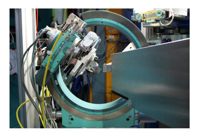
Neutrons can "see" through metal. Therefore neutron diffraction is an ideal method for measuring residual stress inside of components made by additive manufacturing. The image shows a lattice structure in the measurement position on the residual stress diffractometer STRESS-SPEC at the Research Neutron Source Heinz Maier-Leibnitz of the Technical University of Munich. Credit: Dr. Tobias Fritsch / BAM
