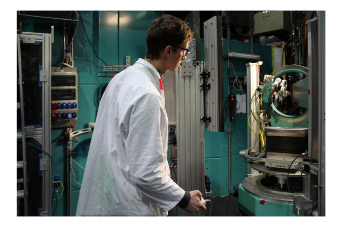
Using the remote control Dr. Tobias Fritsch brings the lattice structure into the correct measuring position in the residual stress diffractometer STRESS-SPEC at the Research Neutron Source Heinz Maier-Leibnitz of the Technical University of Munich. Credit: Dr. Michael Hofmann
