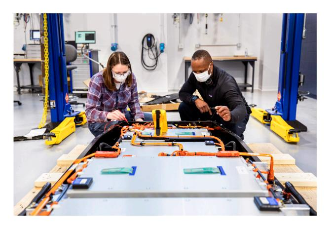
This photo provided by Ford shows Dane Hardware, Ford Motor Co. design and release engineer, and Mary Fredrick, Ford Motor Co. battery validation engineer, measure the voltage of a battery using a digital multi-meter at Ford's Battery Benchmarking and Test Laboratory in Allen Park, Mich., on April 6, 2021. (Ford via AP)
