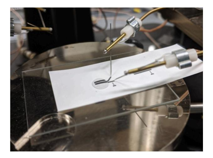
Researchers test a biosensor made out of fully recyclable, printed electronics. The recycling process recovers nearly 100% of the materials used and the materials lose very little of their performance capabilities. Credit: Duke University
