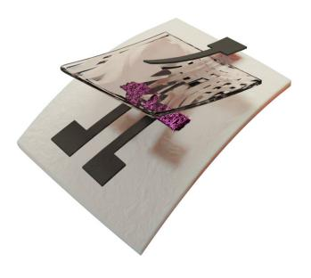
A 3D rendering of the first fully recyclable, printed transistor. Credit: Duke University
