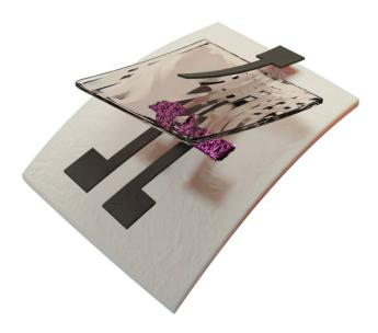
A 3D rendering of the first fully recyclable, printed transistor. Credit: Duke University
