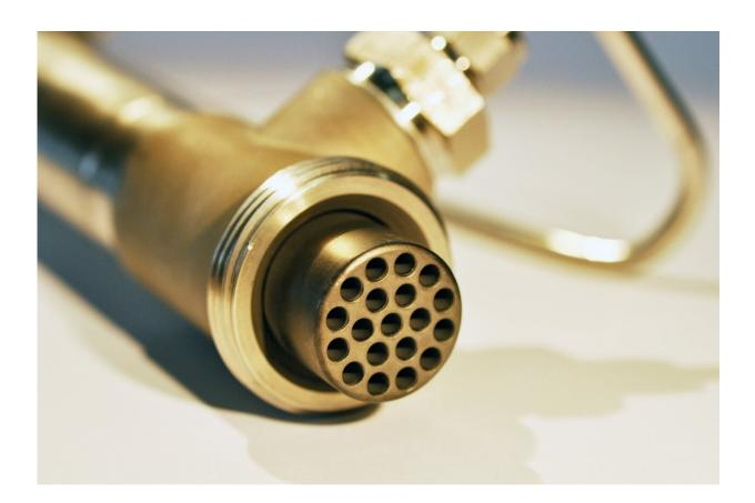
The 19 channels in the carbon membrane enlarge its surface area, and this in turns encourages a higher substance throughput. Credit: Fraunhofer-Gesellschaft
