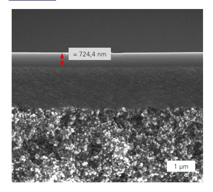
Exposure in the scanning electron microscope: Carbon membrane with a layer thickness of less than 1 micrometer. Credit:
