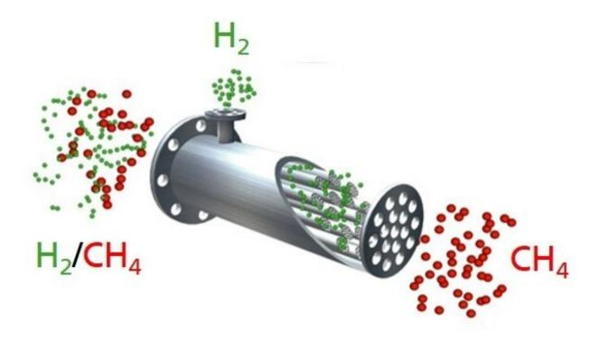
How does a membrane work in principle? The gas mixture is surrendered to the input side of the membrane. The small hydrogen molecules pass through the membranes and the larger methane molecules are held back. Credit: Andreas Junghans GmbH
