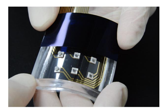
A LED-based haptic film developed by ETRI. Credit: Electronics and Telecommunications Research Institute (ETRI)
