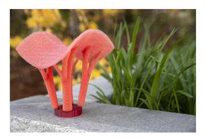
Currently, Paulino and the team are in the prototyping phase, printing structures using a Stereolithography 3D printer with liquid photopolymers as a base. Credit: Candler Hobbs, Georgia Tech
