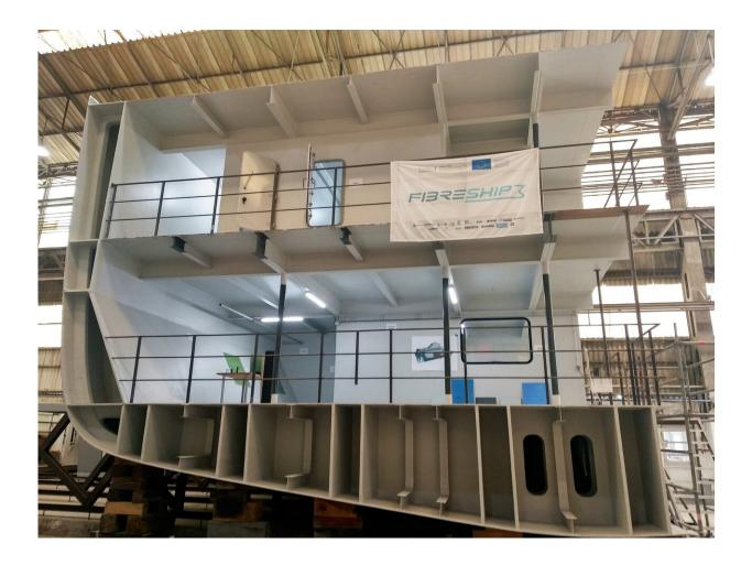
The Fibreship project investigated the feasibility of constructing an entire vessel out of composite materials such as FRP (fibre-reinforced plastic). Credit: TSI
