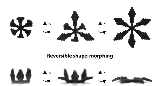
The heterogeneous assembly approach fabricates a flower-shaped soft machine with complex stiffness distribution and reversible shape-morphing. Three of its petals bloomed first in lower magnetic field strength and the rest three bloomed later as the field strength increased. Credit: Max Planck Society
