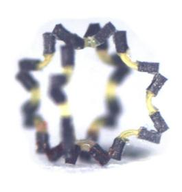
A submillimeter small soft machine that can change its shape. Credit: Max Planck Society
