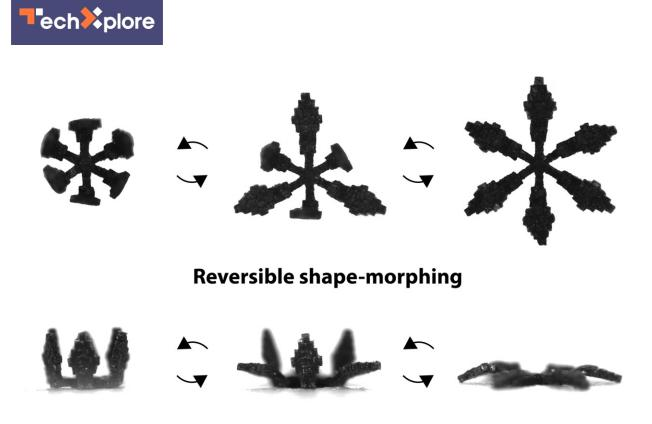
The heterogeneous assembly approach fabricates a flower-shaped soft machine with complex stiffness distribution and reversible shape-morphing. Three of its petals bloomed first in lower magnetic field strength and the rest three bloomed later as the field strength increased. Credit: Max Planck Society
