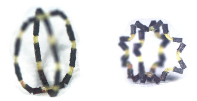
A submillimeter small soft machine that can change its shape. Credit: Max Planck Society
