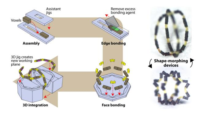
Illustrations of shape-morphing miniature robots fabricated using the heterogeneous assembly platform. Voxels made of multimaterials are freely integrated together to create robots with arbitrary 3D geometries and magnetization profiles. Credit: Max Planck Society
