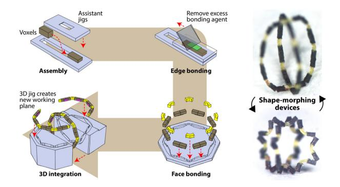
Illustrations of shape-morphing miniature robots fabricated using the heterogeneous assembly platform. Voxels made of multimaterials are freely integrated together to create robots with arbitrary 3D geometries and magnetization profiles. Credit: Max Planck Society
