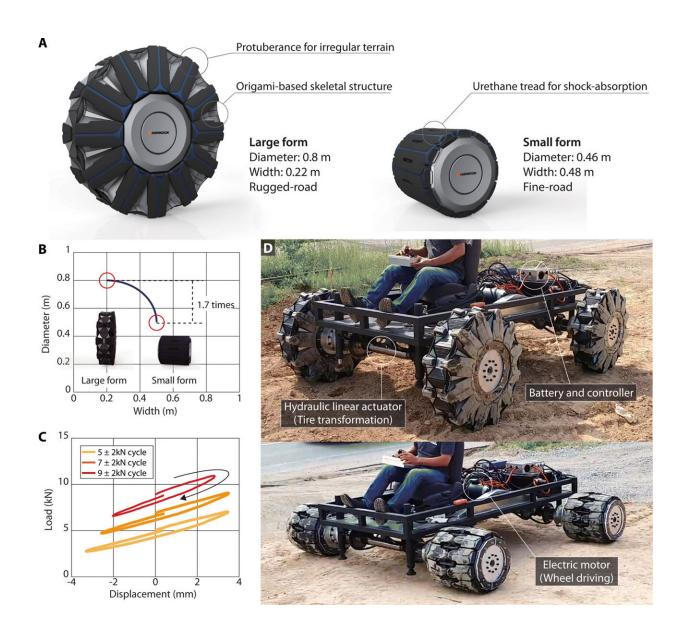
Transformable wheel concept and demonstration. (A) The wheel can be
