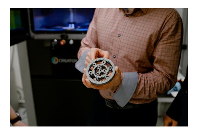
At Alexey Volegov's hands a rotating metal planetary chevron gear, a non-separable system that can only be obtained by 3D printing. Printed at UrFU laboratory. Credit: UrFU/Oksana Meleschuk
