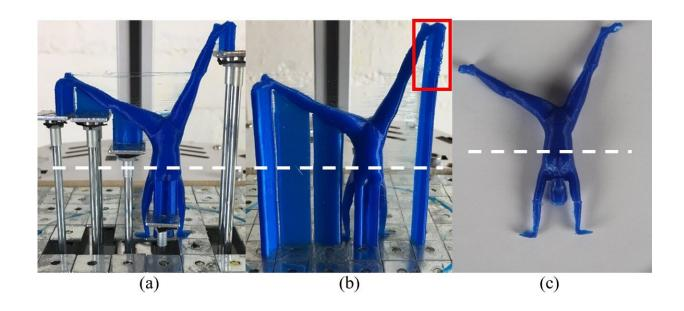
A new dynamically-controlled base for 3-d printing (left) will reduce the need for printed supports (center), cutting wastage and saving time. Credit: Yong Chen
