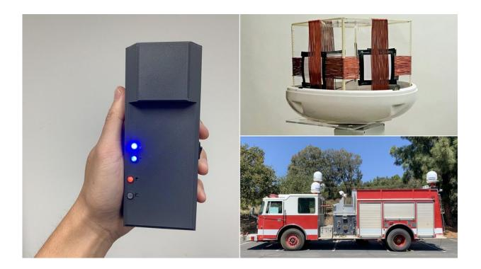
POINTER is composed of a receiver, transmitter, and base station. Clockwise from left: The receiver prototype is worn by firefighters and communicates with the transmitter coil, which was attached to an out-of-service firetruck for testing purposes. Credit: NASA/JPL-Caltech/DHS ST
