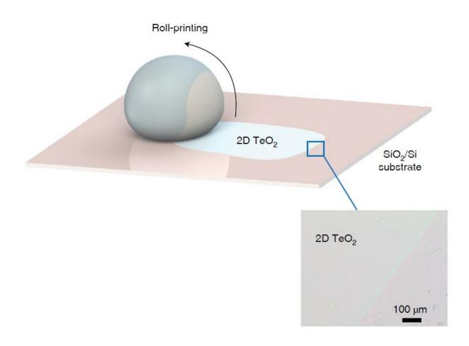
A molten mixture of tellurium and selenium rolled over a surface deposits an atomically-thin sheet of beta-tellurite. Credit: FLEET
