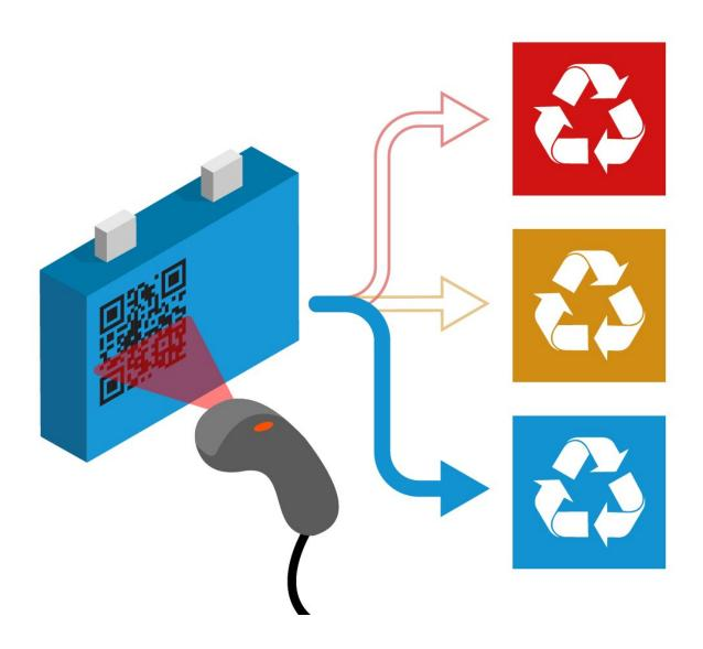
The proposed Battery Identity Global Passport suggests a scannable QR code or other digital tag affixed to Li-ion batteries to identify materials for efficient end-of-life recycling. Credit: Andy Sproles, ORNL/U.S. Dept. of Energy
