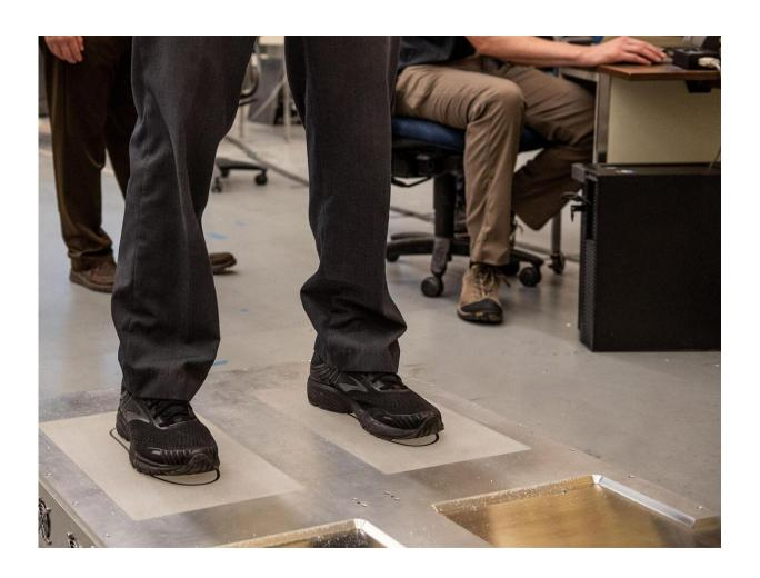
The shoe scanner builds on millimeter wave technology used in passenger scanners deployed at airports to detect concealed weapons. Credit: Photo by Andrea Starr | Pacific Northwest National Laboratory
