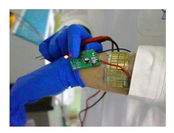
A person wearing the self-powered electric system composed of a TEG band and an LED. Credit: Yijie Liu
