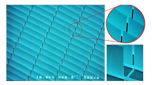
SEM micrograph of vertically standing, flat micromirror array with an inset of magnified area. Credit: Hillmer et al.
